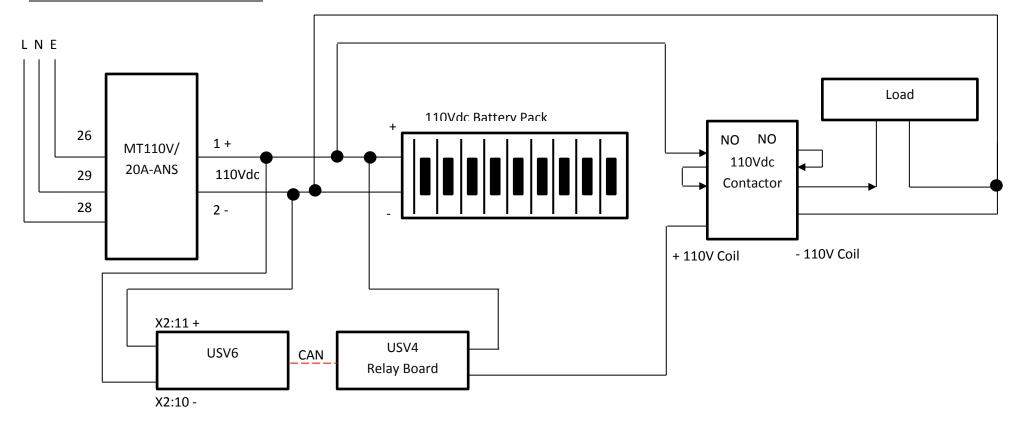
The hysteresis setting on the USV6 is factory set to 5%, but for this application it may need to be increased to around 10% to ensure the battery is not turned on as the battery voltage rises after cut off is reached.
